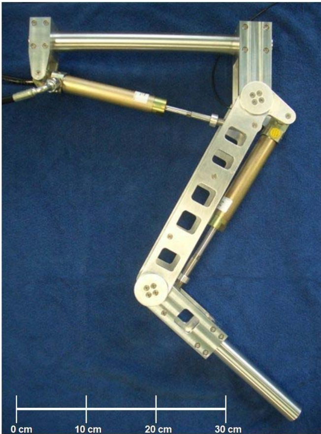
Fig. 5. Picture of HyQ Leg prototype with hydraulic cylinders, without compliant element and foot.
